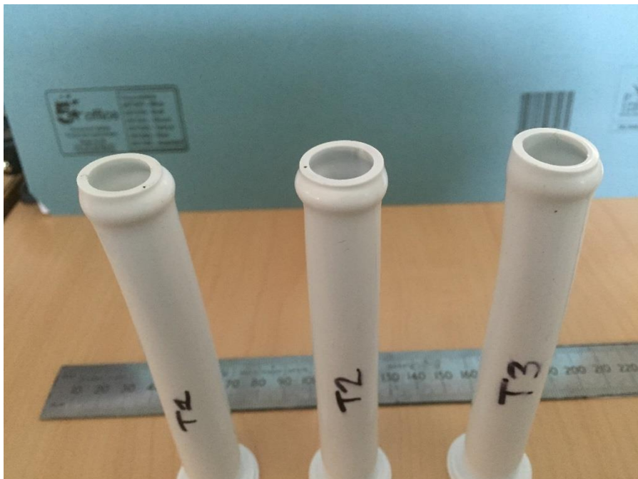
Figure 6 – Compression loads of circa 595 Kg with only minor deformation.
