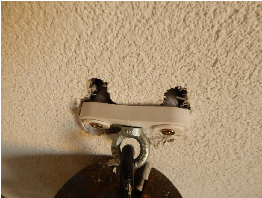
Figure 3 – Fixing failed at this point, (see table 2) notice the cracking of the bracket.
